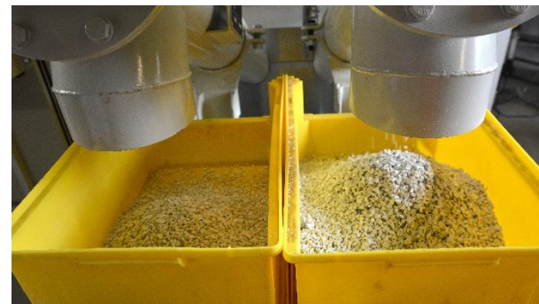
Separated fractions after TBS flake sorting process
